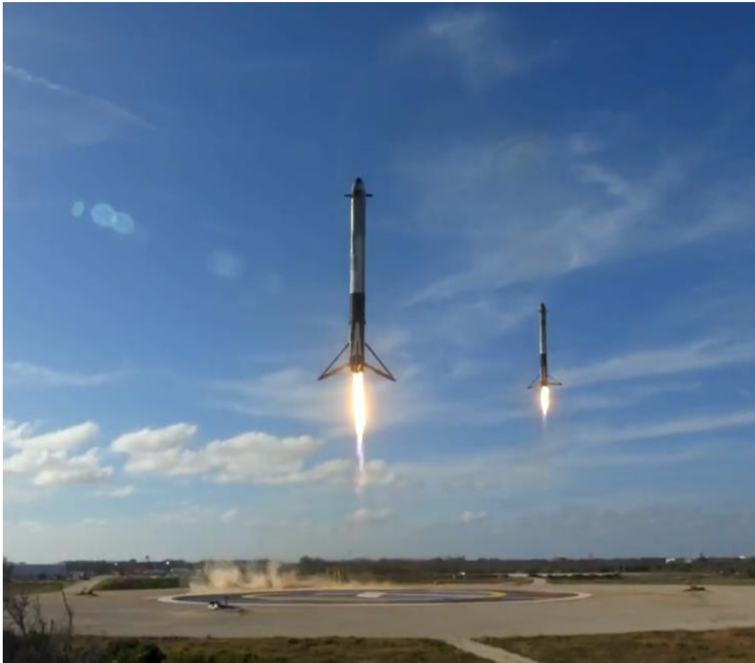
Dual Falcon boosters land following the initial launch of the Falcon Heavy rocket. (Source: SpaceX)
